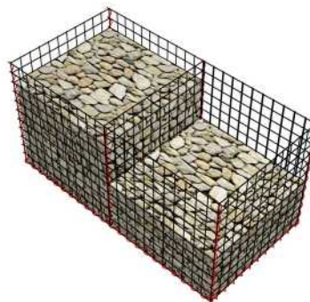
Fill Gabion with Stones
