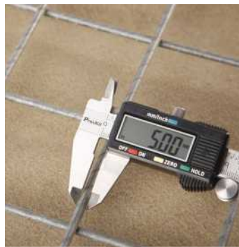
Welded Wire Test
